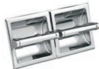
Double Recessed Paper Holder, Chrome Roller, Horizontal, Overall Dimensions 12 1/2" x 6 1/4" - Wall Opening 11 3/8" x 5 1/4" x 1 1/2" 5577
